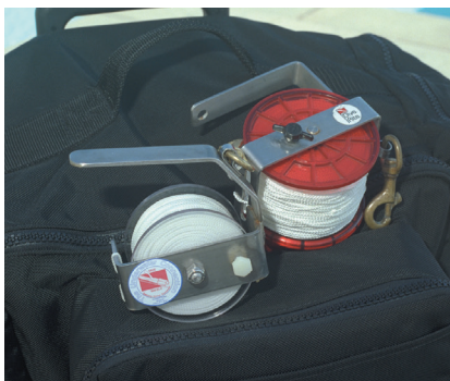
An appropriate reel is compact with ample nylon line to reach the surface. Once inflated, your bag screams upward, so your reel needs to be able to spin smoothly and rapidly, yet allow you to put a bit of drag and control on it.
