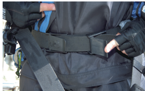
To avoid the possibility of accidental weight belt loss, many tec divers mount two buckles, both of which you must release to get rid of the belt. To them, the slightly slower ditching time is more than offset by the hazard it helps avoid.
