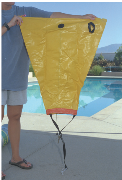
A suitable lift bag is brightly colored, with 45 kg/100 lbs or more lift preferred.
