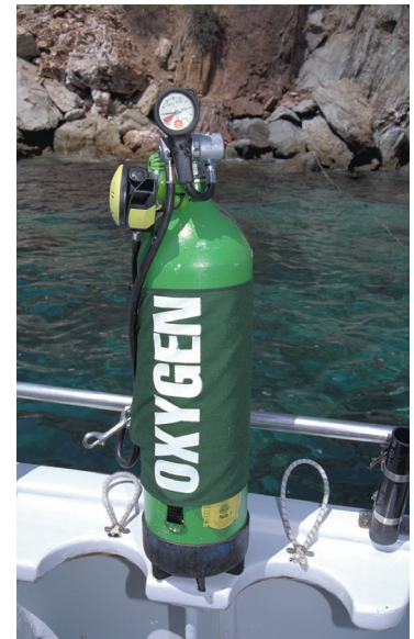
Oxygen cylinder set up as a decompression bottle package. Note the double ended clip used to secure the cylinder at the hip.
