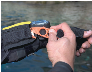
The Z-knife, or hook knife, is a small bladed hook especially suited for cutting fine line. It's commonly mounted via gauge strap on the wrist or harness.
