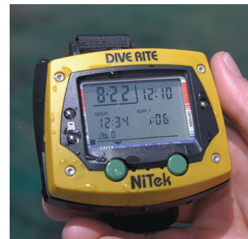
Single gas enriched air dive computers allow you to set for the EANx you're using, usually with up to 40 or 50 percent oxygen. They extend your no stop time and shorten your decompression when using EANx versus air.
