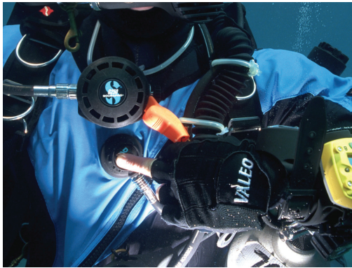
When descending in a dry suit, hold the BCD inflator over the suit inflator. This allows you to inflate both with one hand — the BCD with your thumb and forefinger, and the dry suit with your middle finger. (No impolite gestures intended!)
