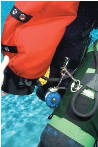
When clipping on to the right hip D-ring, be cautious not to trap your long hose under the cylinder; the hose needs to be below the clip on the D-ring.
