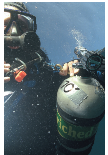
To don a stage bottle, first hold it by the lower clip and secure it to your waist D-ring. Then connect the top clip to a shoulder D-ring.
