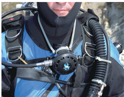
A bungee or surgical tubing “necklace” to hold your short hose second stage is an example of appropriate homemade gear.
