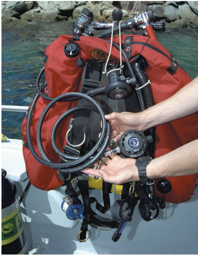
You set up the right post regulator with a low pressure inflator hose to your BCD, and the second stage on a hose about two metres/seven feet long. You set up the left post regulator with the SPG and the second stage on a standard length hose.
