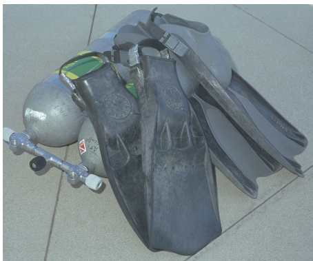
You need full-size power fins with sufficient blade area and flex, like these two well-worn sets. Many fins have strap retainers that keep the loose ends from flopping around (right). If not, you can often reverse them so the loose end routes to the inside or tape the loose ends with duct tape or electrical tape (left).
