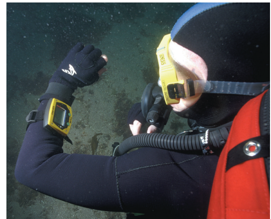
An enriched air dive computer automatically determines EADs as part of its calculations, so you don't need EADs to use it. However, you may still need EADs if your back up deco information employs an air table.
