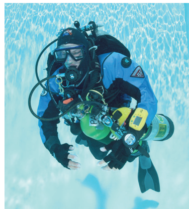
When wearing multiple cylinders on one side, the cylinder that you're breathing from goes on top.
