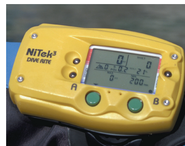
You can set multigas enriched air computers with three or more EANx blends or pure oxygen, allowing the computer to alter your decompression and oxygen exposure when you switch from one gas to another during the dive. They can extend your no stop time, accelerate your decompression based on the gas switches, and track your oxygen exposure.
