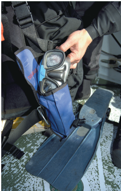
A suitable spare mask is as small and compact as possible. The usual carrying place is in a compact harness pocket on the waist band all the way back, behind the waist D-rings.
